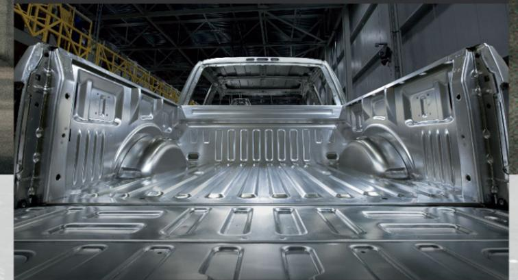
EXTREME STRENGTH. The F-150 body and cargo box are constructed with high-strength aluminum alloy, which is hardened through heat treating.
